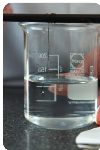
▲ A seed crystal can be used to grow a larger crystal by suspending it in a saturated solution
